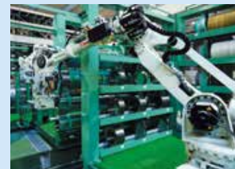
Slitting line's automated blade changer
