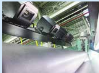
Automated defect detection equipment installed on the 1600-millimeter leveling line as part of our efforts to improve customer satisfaction
