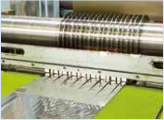
Expansion arbor for blade vibration control
