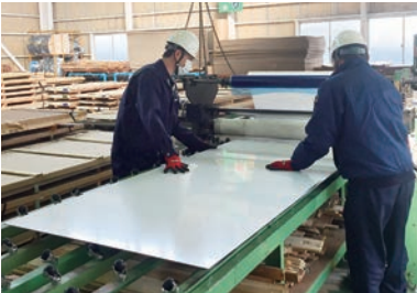
Plastic film laminator handles both surfaces
