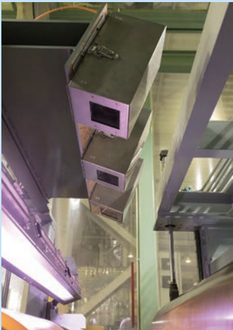
Dual surface inspection equipment
