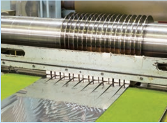
Expansion arbor for blade vibration control
