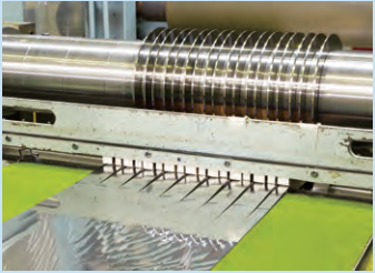
Expansion arbor for blade vibration control
