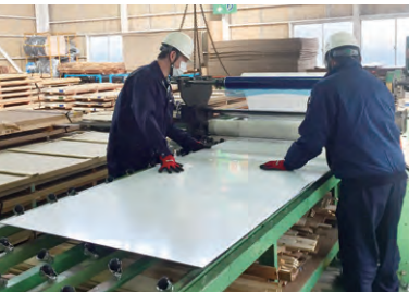
Plastic film laminator handles both surfaces
