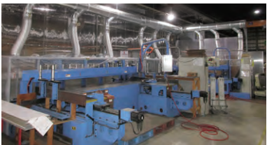
Right-angle milling machine able to handle three-meter lengths
