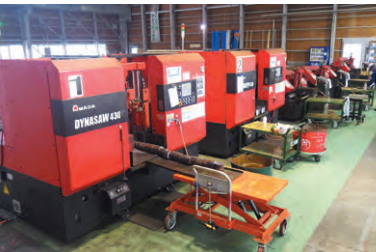
Cutting in diameters from 10 to 430 mm possible
