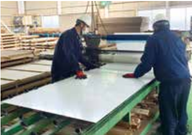
Plastic film laminator handles both surfaces
