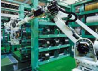
Slitting line's automated blade changer
